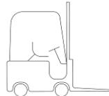
The products shall be handled with a forklift; insert the forks under the pallet, lift the products, and bring them to the place of installation, and make sure the load is not unbalanced.
